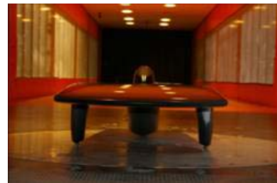
Figure 2 – 1/3 scaled model in the wind tunnel
